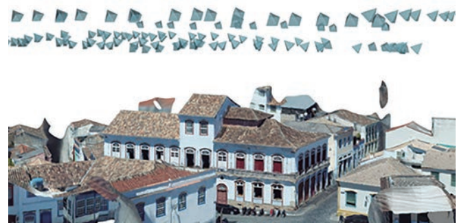
Figure 6. Urban scale 3D mesh and photo captures location above the Baroness Solar building. Source: Silva (2017).
